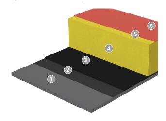
The pre-formed system comprises Im x 0.5m C50 tiles bonded to substrate and site applied D2004 phenolic laminate.
